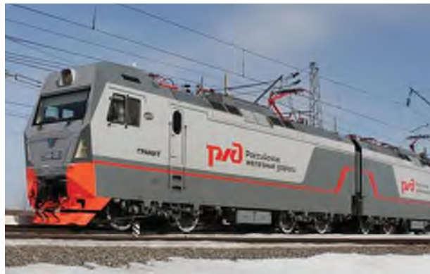
Fig. 3 The appearance of 2ES10 Electric Locomotive. Source: RIA Motor
