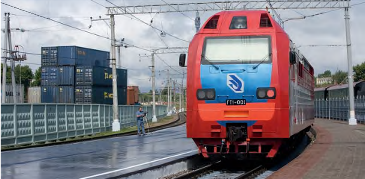
Fig. 1 Gas turbine locomotive GT-1
