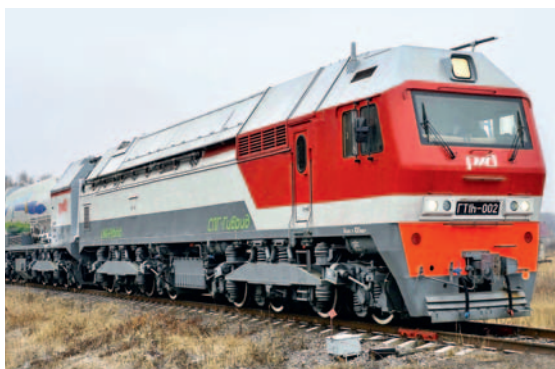
Fig. 5. Gas-turbine locomotive GT1h-002 based on the underframe of diesel locomotives TEM7A
