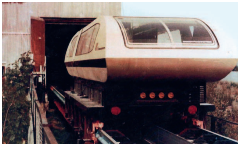
Fig. 4. Carriage TP-05 with electromagnetic levitation and linear electric drive at the experimental proving ground in Ramenskoye
