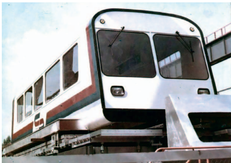
Fig. 3. The first Soviet carriage with magnetic levitation system and linear electric drive
